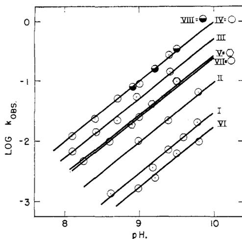
Fig. 1.—Plots of the logarithm of the observed first-order rate constants ( $\log k_{\text{obs}}$ ) for hydrolysis obtained at  $78^\circ$ ;  $\mu = 1.0 M$  vs.  $pH$  for various esters studied.
