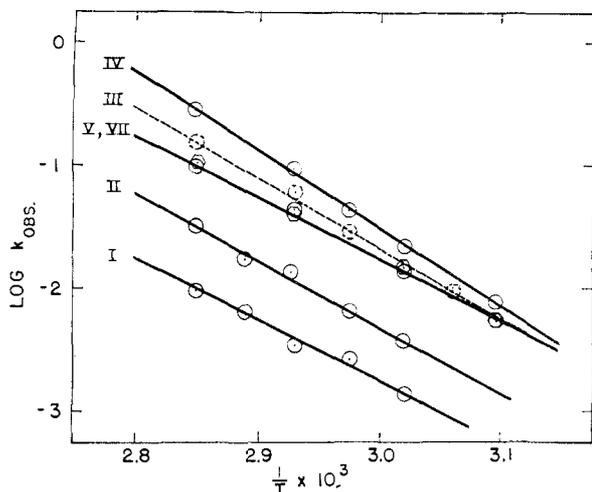
Fig 2.—Plots of the logarithm of the observed first-order rate constant ( $\text{min.}^{-1}$ ) for hydroxide ion catalysis of the esters I through V and VII. The values of  $k_{\text{obs}}$  were obtained at constant  $\text{pH}$  values of 9.5 for I, II, V and VII and 9.4 for III and IV.  $\text{○} = \text{V}$ ,  $\text{○} = \text{III}$ .
