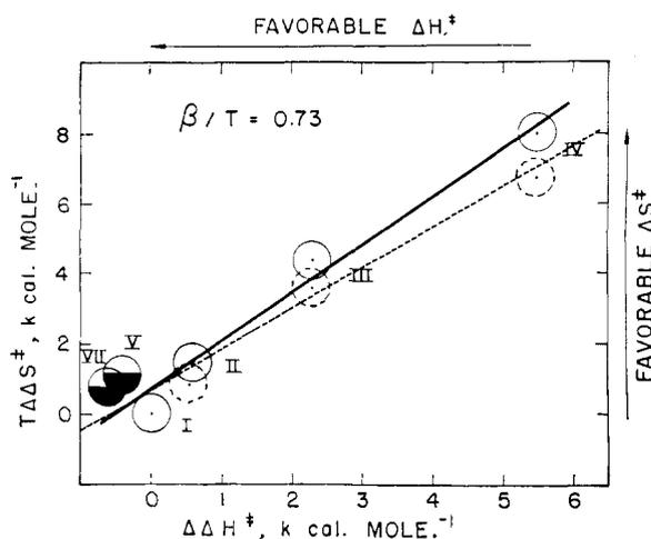
Fig. 4.—Plot of  $\Delta\Delta H^\ddagger$  vs.  $T\Delta\Delta S^\ddagger$  at 78° for the esters I through V and VII. Cyclopentylacetate was employed as the standard. The dashed line represents the same plot derived from data obtained by extrapolation of Fig. 2 to 25° and calculation of the activation parameters at this temperature. The circles were drawn with a radius of  $\pm 250$  cal./mole in  $\Delta\Delta H^\ddagger$ .
